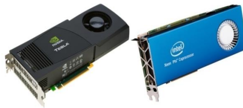
Accelerators / Coprocessors high compute density, high performance/watt >1 TFlop DP on a chip
